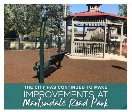
This year a new overlay material called Flexipave was installed around the fountain and shelter areas. The product is made from 100% recycled shredded car tires that are mixed with small stones and bound with an adhesive product. Nearly 7,000 tires were recycled on this project.
